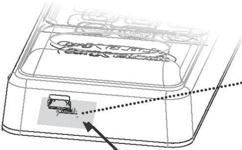
USB Port for direct connection to LockView software
