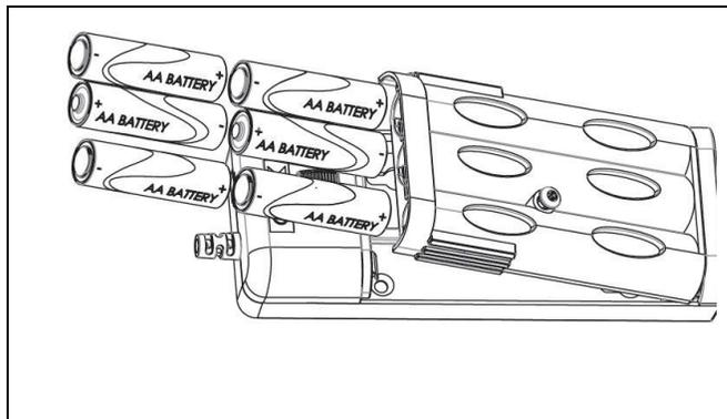
Warning: install the batteries as shown in the battery compartment. Polarity (+) or (-) must be correct. Replace batteries as a set. Always use new batteries when replacing the old set. Do not combine a used battery with a new one. Only use premium alkaline batteries; do not mix battery types.
