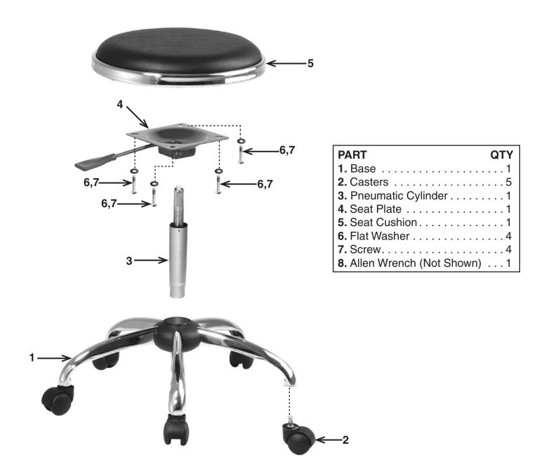
Remove all parts from carton, separate by part numbers indicated on parts list, and verify part quantities.
