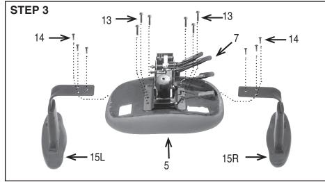
13. Phillips Head Screw......6 14. Mechanism Screw . . . . . . . . . 6 15. Arms Left (15L) Right (15R) . . . . 2 16. Back Support (Pre-Installed) . . . . 1 17. Allen Wrench (Not Shown) . . . . . 1
